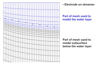
Figure 47. Mesh used to model water layer.
