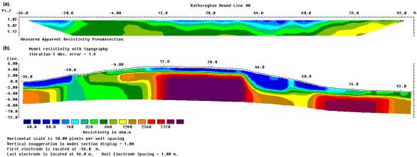
Figure 37. Example of the model for the Rathcrogan Mound data set. (a) Measured apparent resistivity pseudosection. (b) Inverse model section with topography.
