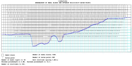
Figure 31. Arrangement of model blocks and the water bottom boundary for an arrangement with the water layer incorporated into the inversion model.
