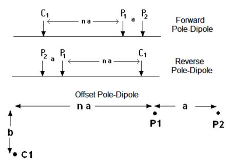
Figure 45. Normal, reverse and offset pole-dipole array arrangements.
