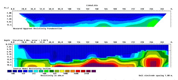
Figure 32. Inversion model for the survey with floating electrodes along the along the São Francisco River in Brazil. The thin black line indicates the water bottom boundary.
