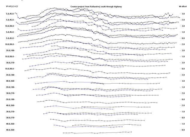
Figure 25. Plot of a multiple gradient array data set in the form of profiles using exact pseudodepths for the CROMER2.DAT file.
