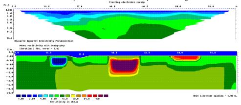
Figure 30. Example of inversion model with a fixed water layer. The inversion results of the WATER\_FLOAT.DAT data is shown where the resistivity water layer (represented by the top blue layer in the model section) is fixed and model extends from below the water bottom.
