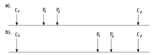
Figure 26. Two different configurations of the gradient array with the same pseudodepth but with the potential electrodes at different sides of the array. Gradient array configuration with (a) right parity and (b) left parity.
