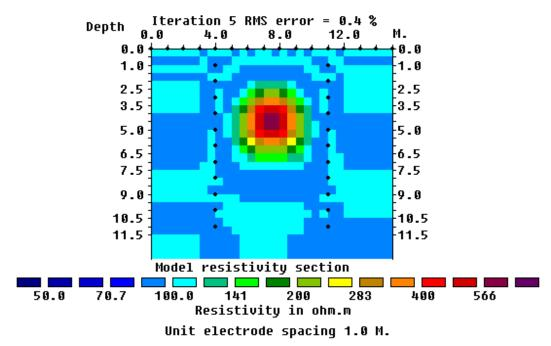
Figure 12. The model obtained after the inversion of the BOREHOLE.DAT data set. The option to use finer blocks with half the size of the spacing between the electrodes was used.
