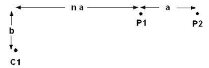
Figure 6. Arrangement of electrodes for the offset pole-dipole array.
