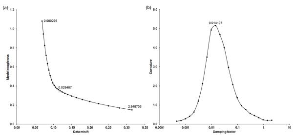
Figure 23. Example L-curve plot to determine the optimum damping factor for the BLUERIDGE.DAT data set. (a) Variation of model roughness with data misfit for a range of spatial damping factor values (a few values are shown near the corresponding points), (b) variation of the curvature of the L-curve with the damping factor.
