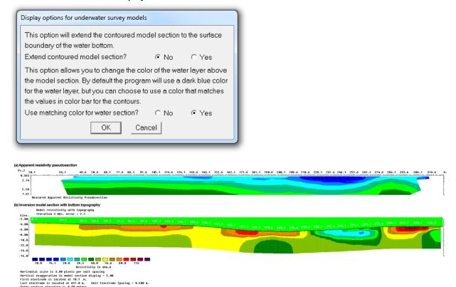
Figure 42. Example of underwater survey. (a) Apparent resistivity pseudosection. (b) Model section with topography. Note the contoured model plot has been extended upwards to the water bottom interface, and the color of the water layer matches the contour scale used for the resistivity sections. This example is from an underwater riverbed survey by Sage Engineering, Belgium.
