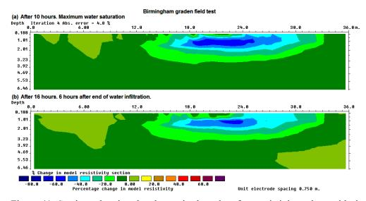
Figure 41. Sections showing the change in the subsurface resistivity values with time obtained from the inversion of the data sets collected during the infiltration and recovery phases of the study.
