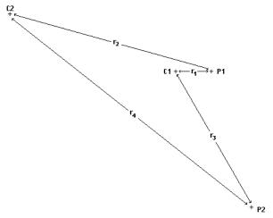
Figure 9. A schematic diagram of the arrangement of the electrodes in an actual field pole-pole measurement.
