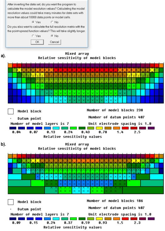
Figure 35. Two arrangements of model blocks using the extended model and sensitivity values methods. The arrangement of the model blocks used by the program for the inversion of the MIXEDWS.DAT data set using (a) the default extended model and (b) a model generated so that any single block the does not have a relative sensitivity value that is too small.
