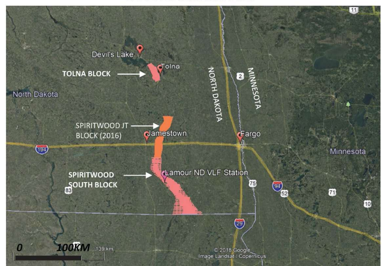
Figure 1 - Spiritwood South and Tolna survey location map, showing 2018-19 VTEM ET survey to the south and north, respectively consisting of 2433 and 566 linekm at 1-5km line spacing, and 2016 VTEM Plus survey (Legault et al., 2017b) in the center, consisting of 1950 line-km at 0.5-5km spacing (after Legault et al., 2019ab).
