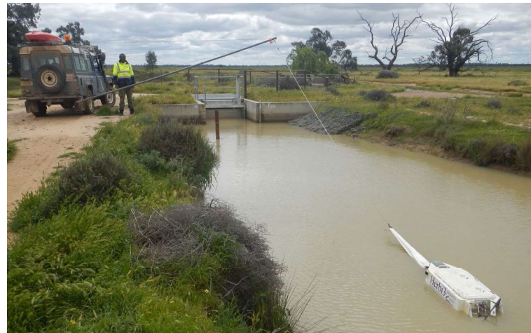
Figure 2: HERBI survey using a fold-in boom extending from the side of a vehicle and occasional detachment and manual manoeuvring.
