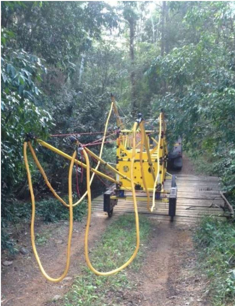
Figure 11: AgTEM-cart booms fold backward permitting width reduction to 1.8m. Signal lights and reflectors facilitate travel in traffic.
