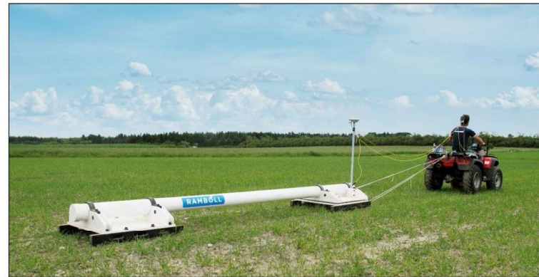
Figure 1 System setup for optimal operation. The DUALEM421-S sensor is mounted in the PVC pipe, Ramboll.
