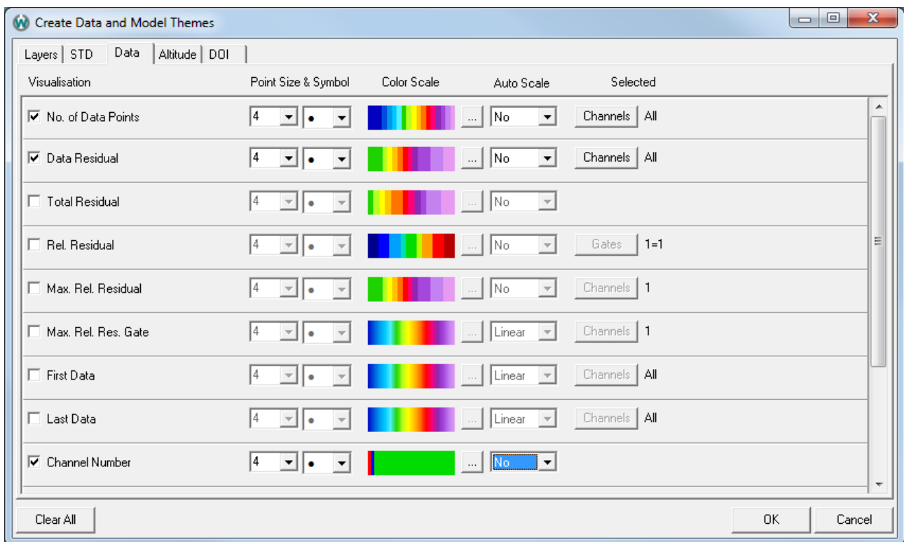
Figure 6.3: The model quality setup. Use the F1 wiki help to read more about the setup.
