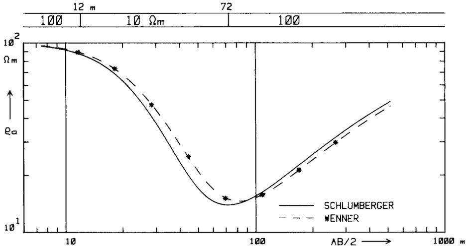
FIG. 2. Schlumberger and Wenner sounding curve for the model in the top of the figure, and Wenner data (\*) as obtained with  $AB/MN = 3$  from Figure 1.
