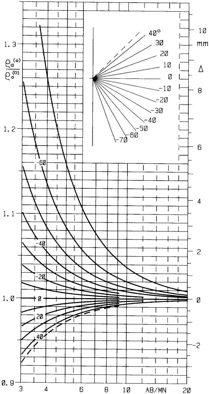
FIG. 1. Ratio of apparent resistivity  $\rho_a^{(a)}$  (distance  $a$  between potential electrodes  $M$  and  $N$ ) to apparent resistivity  $\rho_a^{(0)}$  for a Schlumberger configuration ( $a \rightarrow 0$ ) versus the ratio  $AB/MN$  for several slopes of the Schlumberger curve.
